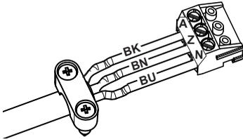
4. Plug in the connector with new cable and fit the strain relief.
