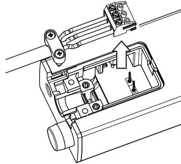
3. Disconnect the cable from the connector and connect the new connection cable using wire end ferrules.
